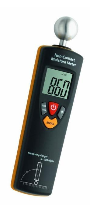
The Humidcheck Contact Moisture Measuring Instrument is able to measure the moisture levels of wood and construction materials by touching the item with the silver metal ball. The depth of the measurement is 40mm.
